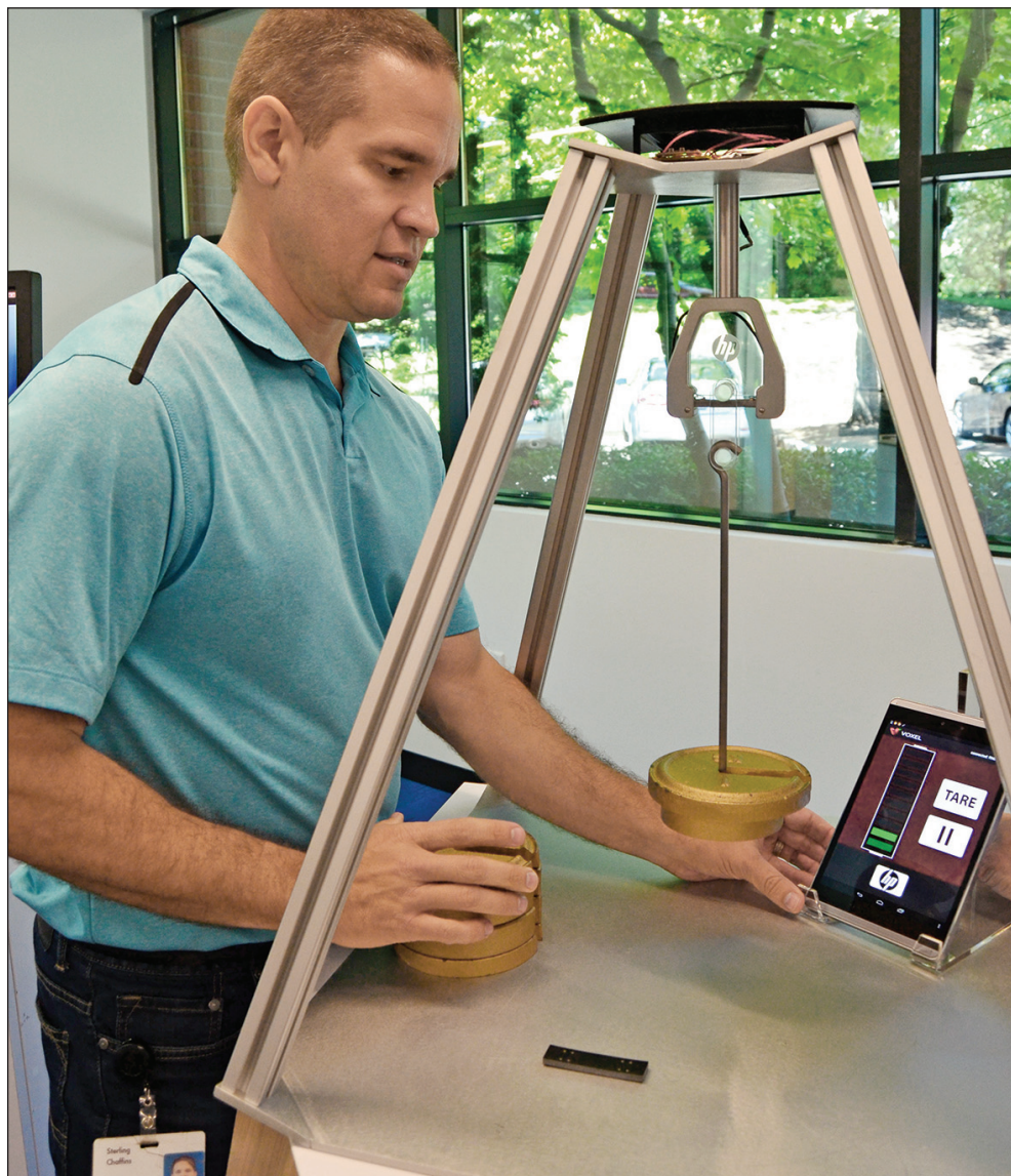
Sterling Chaffins adds weight to a 3D printed piece with embedded circuits that track the weight in real time on a tablet as he adds it.
