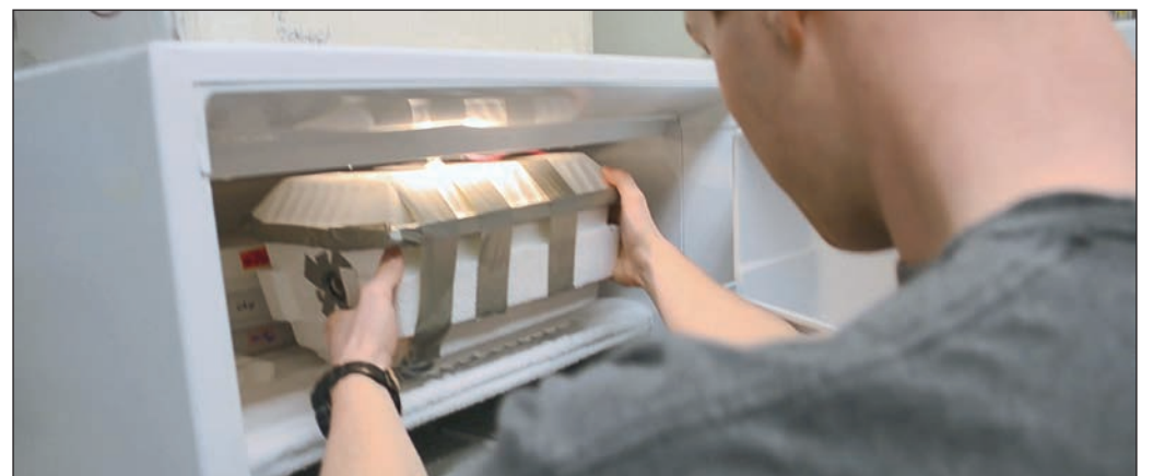
The spacecraft Near Space Venture used needed to be able to withstand temperatures as low as minus 60 degrees F, so it was tested it in a minus-110-degree freezer. Here, Logan Rooper places the spacecraft in the freezer.
